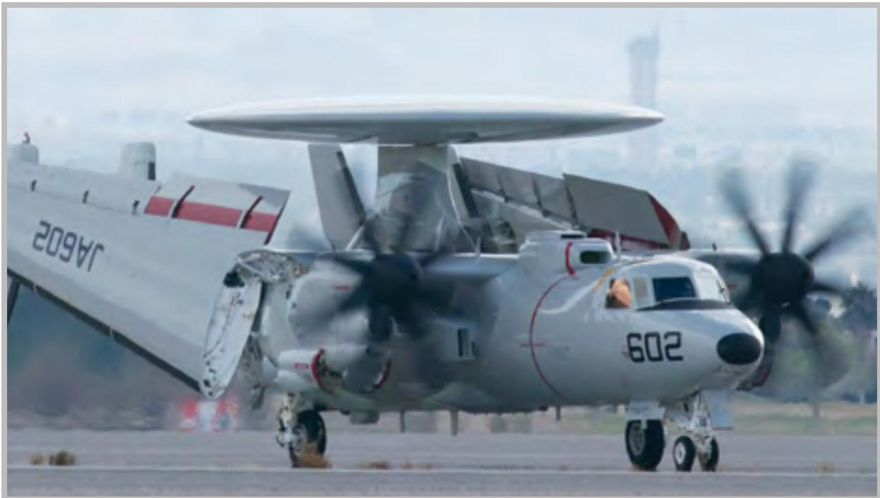
The 360-degree, continuous scan operations unique to the E-2D radar also permit more tactical flexibility during patrol missions. For instance, the E-2D can shift its flight route yet still maintain backward-looking radar coverage as it repositions.
